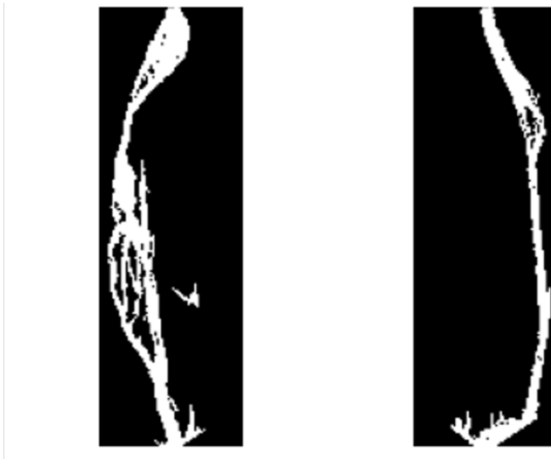
Figure 3.3: Most dissimilar morphologies across the experiment according to both MHD and Dice. The left panel shows a slightly more laterally expanded, multi-thread pattern; the right panel shows a narrower, single-thread channel.
